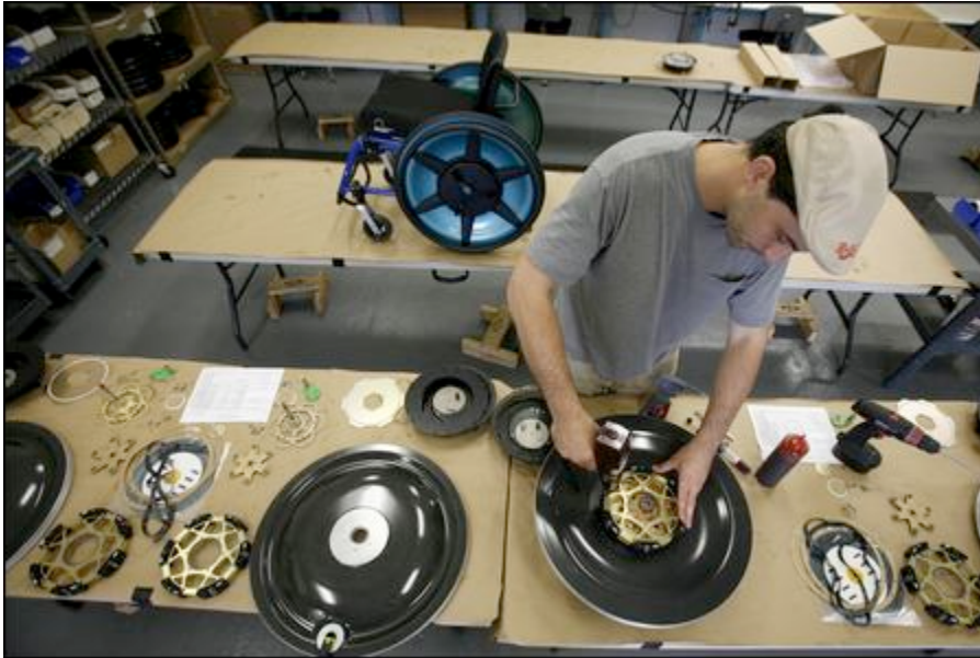
Jason Casatelli, production supervisor at MagicWheels, assembles a wheel equipped with the company's gear mechanism. A finished wheelchair is at center left. (Paul Joseph Brown / P-I Photos)
