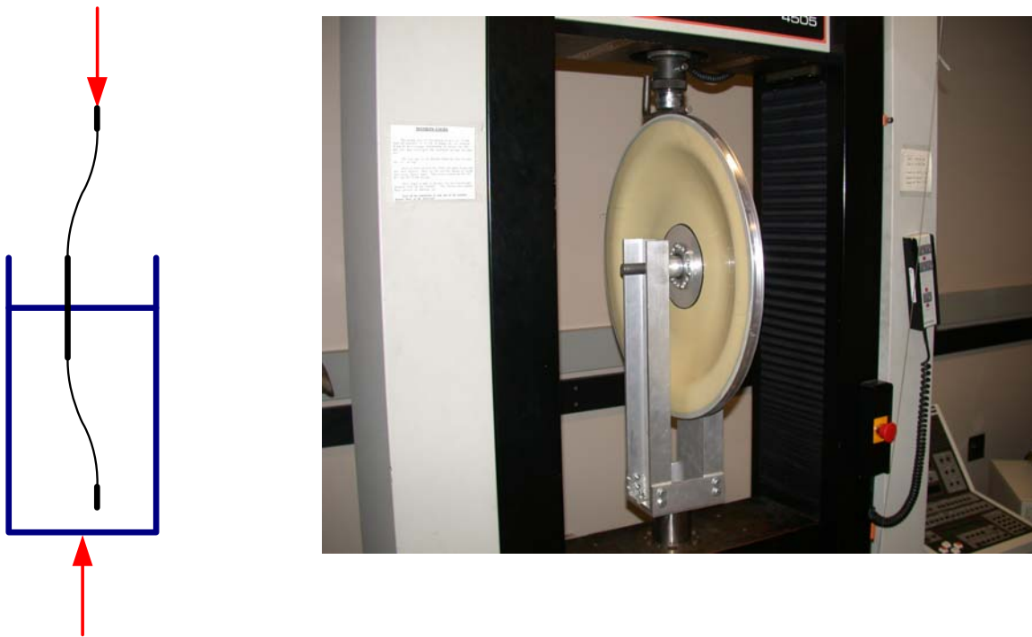
Figure 1: Photo and schematic of radial loading test
