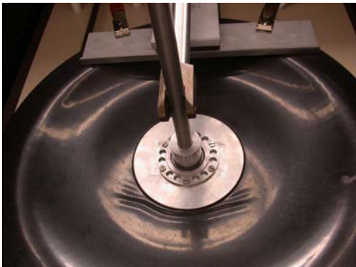
Figure 3. Wrinkling of carbon fiber composite wheel while under load. No wrinkles were detectable after load was removed.
