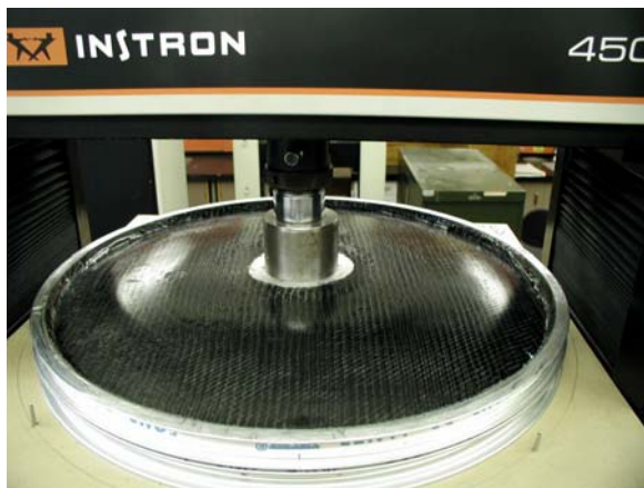
Figure 1: Photo and schematic of axial loading test
